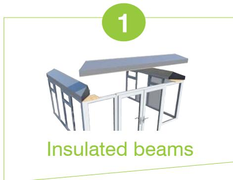
1. A patented box eaves beam, filled with EPS beads as used in cavity insulation - that forms the soffit structure - approx 380mm front to back depth.
