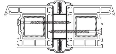
Mullion as a wind post:- the size of the mullion depends on the height of the frame. With full height frames (2100mm) the mullion needs to be the full front to back depth of the window frame and at least 20mm wide.
