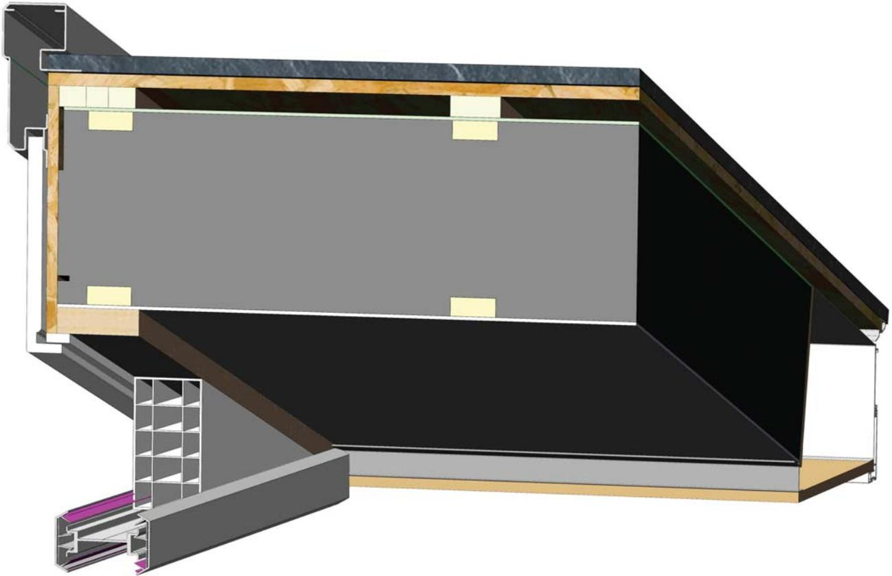
A gable tie beam is supplied on every gable project the tie beam has an offset of 21mm and the underside lines up with the top of the existing frames – see illustration.
