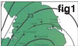
Use figure 1 to check the wind speed at the location (in this case its 23 m/s which translates on table 1 to 0.68 kN/m<sup>2</sup>). From figure 2 check the snow load at the location (which is 0.6kN/m<sup>2</sup>).
